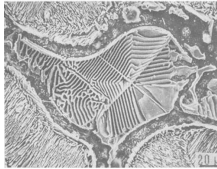
Figure 11. Morphology of eutectic M_6C carbides [48]
