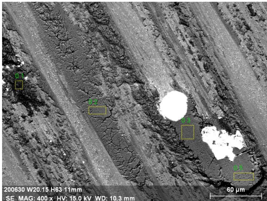
Figure 86. Composition zones of different parts of the mix of debris and tribolayer present on W20.15 H6.3 8mm
