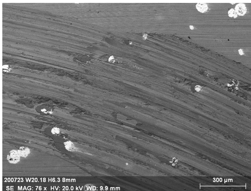
Figure 90. Track width change overview along with a tribolayer overview
