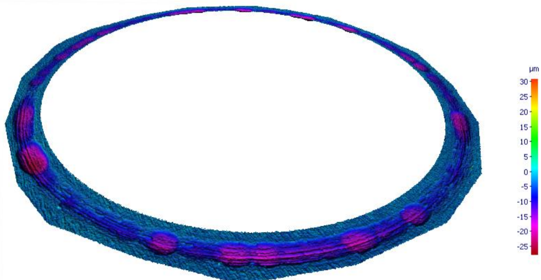
Figure 67. W20.15 F1.3 11mm worn track 3D overview
