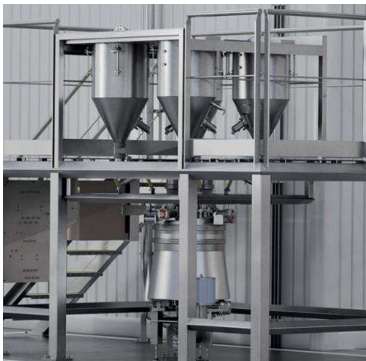
Figure 52: Station de dosage des micro ingrédients Gashor
