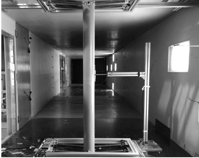
Figure 4.1: Experimental test rig used in the wind tunnel of the University of Liège
