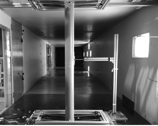
Figure 16: VIV Test Rig [72]
