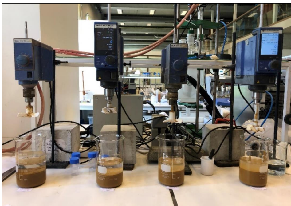
Figure 25: Jar test set-up used for pH optimization
