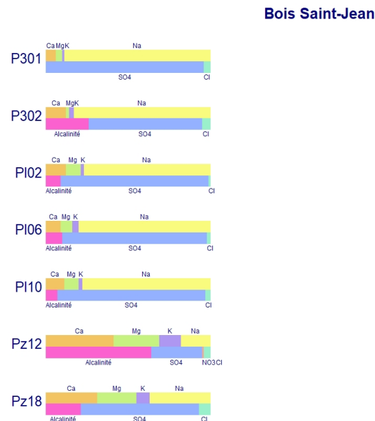
Figure 11. The mineralisation of the water samples, with their respectively cation and anion composition.
