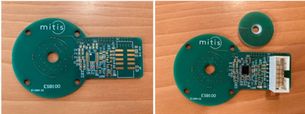
Figure 4.28 – (a) PCB's received from the manufacturing company (b) Assembled card
