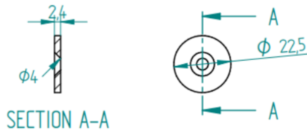
Figure 4.15 – Mechanical design of the target
