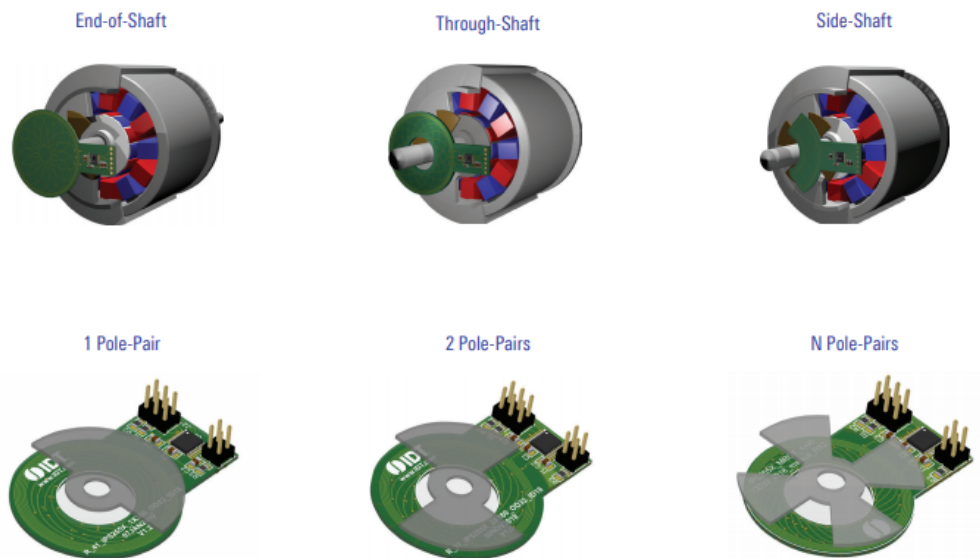
Figure 4.8 – Up : Design with respect to the shaft configuration. Down : Target design with respect to the number of pole pair [20]
