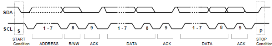
Figure 5.3 – General data transfer I^2C protocol[22]
