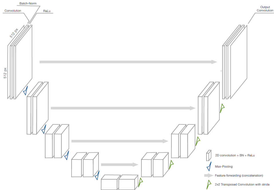
Figure 2.9: The FCNN architecture (Source: [Sakinis et al., 2019]).
