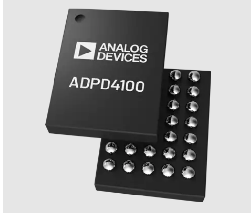
Figure 2.3: ADPD4100 in its WLCSP package[45].
