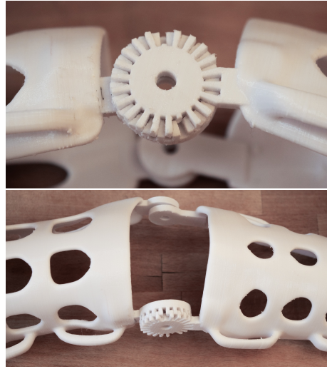
(b) Blocking hinges printed vertically in PET. Supports in PLA were removed. The missing teeth are noticeable and the two parts do not fit easily.
