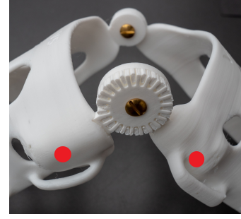
(b) Two binding screws are visible and the two additional screws would be placed on the red points to fix the sliding hinge in the splint.
