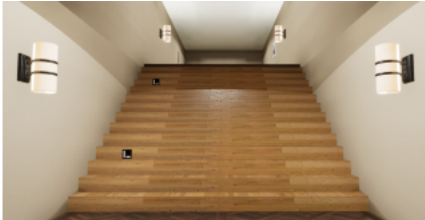
Figure 6.18: Example of a staircase with markers placed at different steps to help the drone crossing it.
