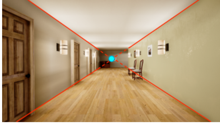
Figure 6.2: Example of a vanishing point (in blue) in a corridor image. The parallel lines (in the real world) are represented in red.
