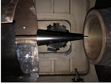
Figure 9: 7.4°-half-angle, 3.5-mm-nose-radius conical model injected in test section.
