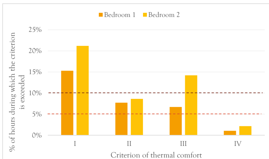
Figure 19 – Comparison of the four thermal comfort criteria in the bedrooms for the year 2100 of the medium simulation.
