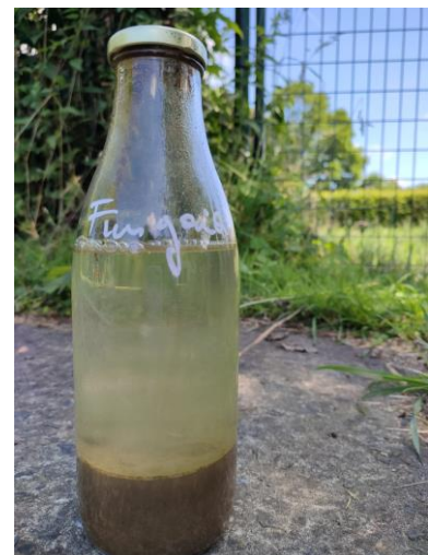
Figure 5 – Test de sédimentation
