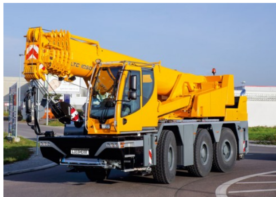
Figure 4 - Grue automotrice (LTC 1050-3.1)
