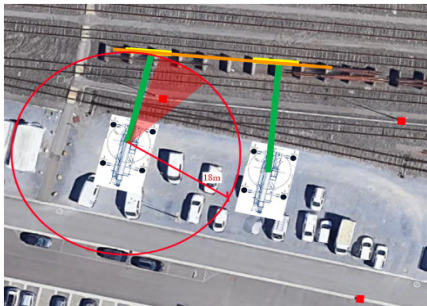
Figure 14 - Rayon max - GMK 3060 (Source : Mincke F., 2021)
