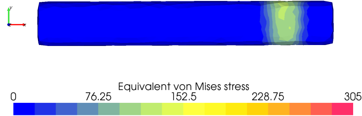
Figure II.26: Equivalent Von Mises stress field of screw 3, mesh density factor m = 0.7 .
