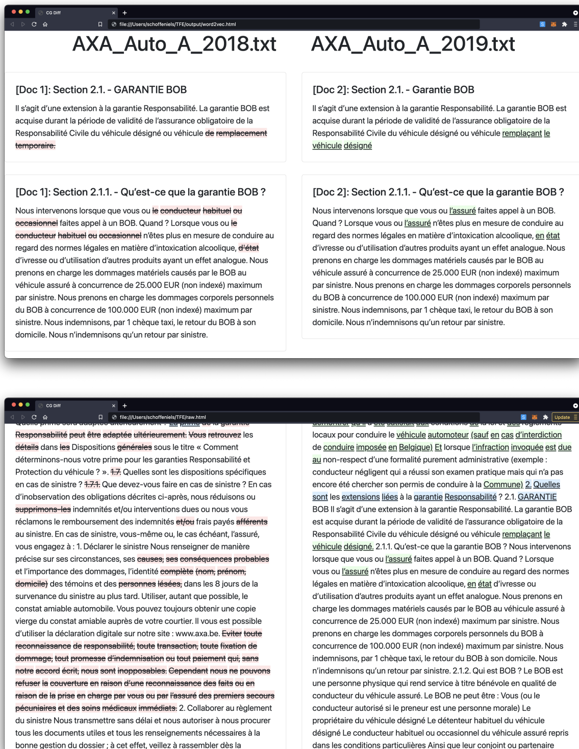
Figure A.3: Comparison of using the comparison module on sections (at the top) and on the complete documents (at the bottom). The output of the tool implemented is cleaner, more readable. Using the comparison module on the complete document makes it hard to find to which modifications from the left side correspond the one from the right side.
