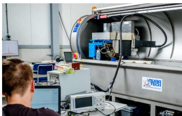
Figure 26. LIBS-XRF core scanner prototype developed by SPECTRAL Industries and Avaatech's XRF core scanner (Dalm et. al. 2019)
