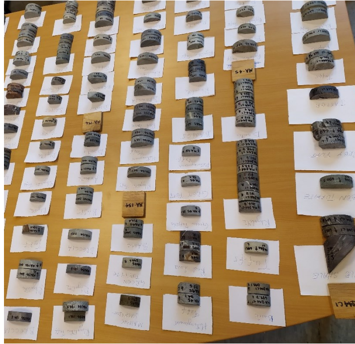
Figure 27. Rock pieces sliced from the main drill-core samples.
