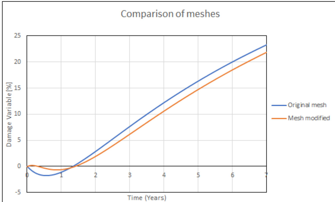
Figure 4.29: Corrosion comparison between original mesh and modified mesh
