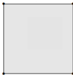
Figure 3.5 Element of 4 nodes (Quad4)
