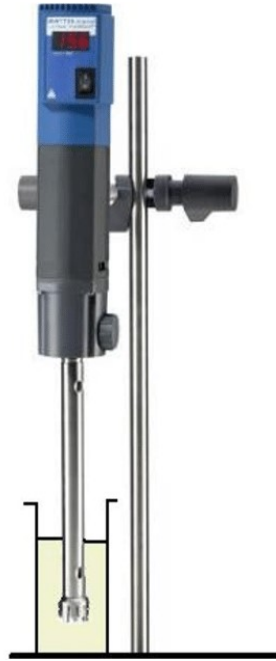
Figure 56: Rotor Stator Homogenization [29]
