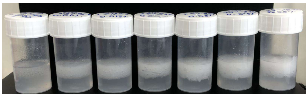
Figure 52: Macroscopic Images of emulsions prepared by 1% BIS large microgels using large axis and PDMS
