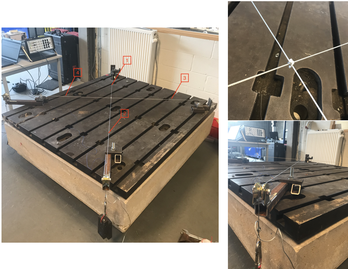
Figure 3.7: Assembly of the cross-cables network set-up
