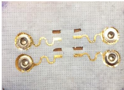
Figure II.7: Gold electrodes on a PET substrate embedded into medical tape (from [41])
