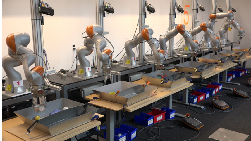
Fig. 3.2 Original data collection setup from QT-Opt ( Kalashnikov et al., 2018 ). It can be seen that the surroundings of the robot as well as its model are perceived by the over-the-shoulder camera.
