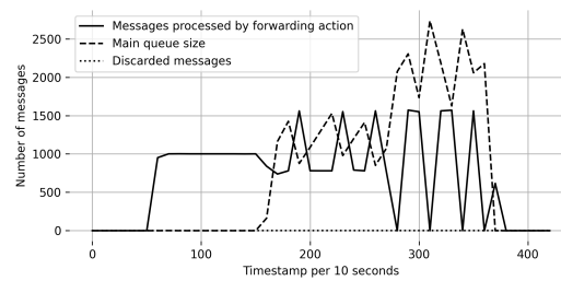
(d) Small profile internal counters with a minimalist configuration. The maximum size reached by the queue is 2,735 ( \sim 6\% ) and the average 757 ( \sim 1.5\% ).
