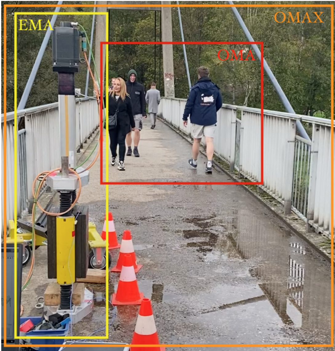
Figure 1: Illustration of the OMAX method being a combination of EMA (uses only artificial forces) and OMA (uses only ambient forces). In this figure, those forces are represented by a shaker and pedestrians respectively.
