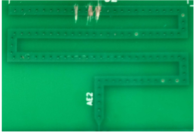
Figure 5.20: Practical meander antenna cut.
