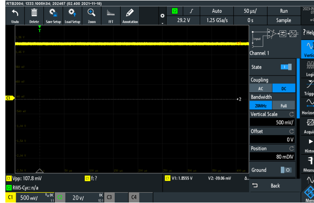
Figure 6.4: E-peas output voltage with no load.
