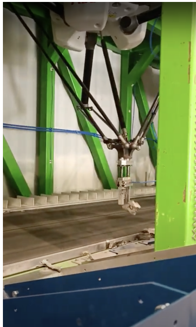
Figure 4.5.: Throw with the Flexpicker using TD3 algorithm.
