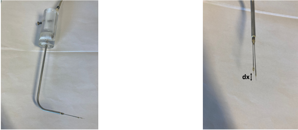
FIGURE 3.5: Double-tips conductivity probe.
