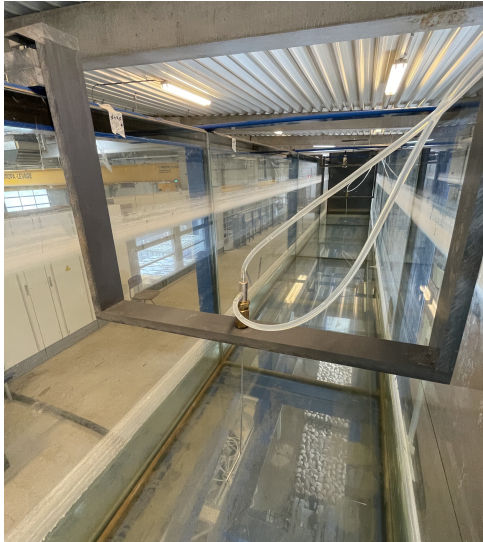
FIGURE 3.12 – Installation des tubes de Pitot
