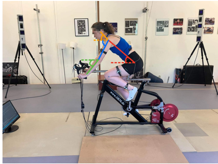
Figure 4.16: Final angle definition : the neck angle is in orange, the shoulder angle is in blue, the elbow angle is in green and the hip angle is in red.
