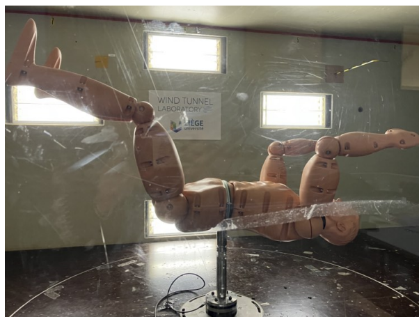
Figure 2.2: Helmets testing set up with the mannequin.
