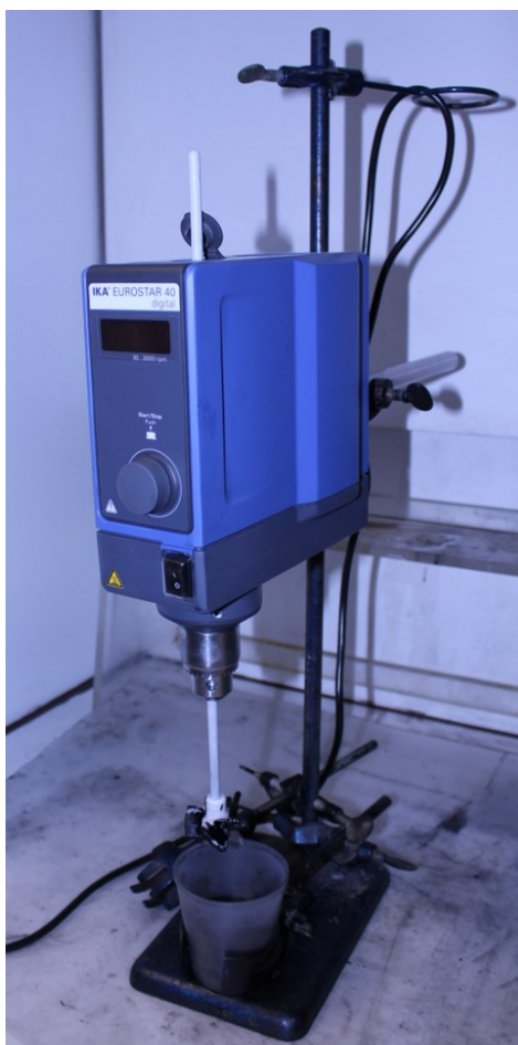
Figure 4: Mechanical stirrer and slightly inclined four-bladed propeller.
