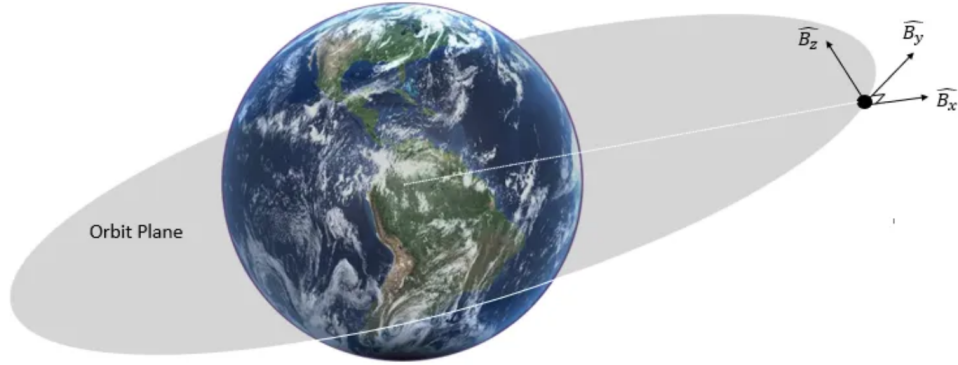
Figure 1.4: Spacraft Body-Fixed Frame Representation [30].
