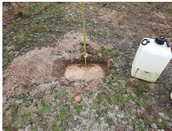
FIGURE 1.22 – Essai Matsuo (Sond&Eau, 2023).
