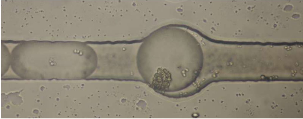
Figure 10.9: Experimental picture showing the formation of a spheroid within the dropspot chip. The height is set at H = 80 [ \mu\text{m} ]. The approximate volume of the droplet is estimated to be 1000 [pL].
