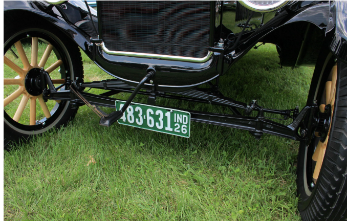
Figure 3: Front suspension of the Ford T[12].
