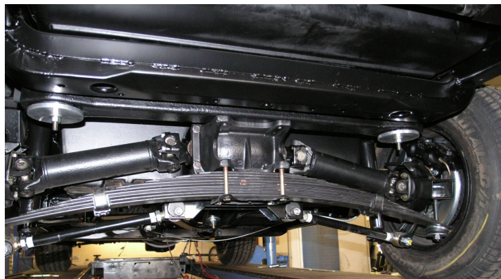
Figure 4: Rear suspension of the Chevrolet Corvette C2 [14].
