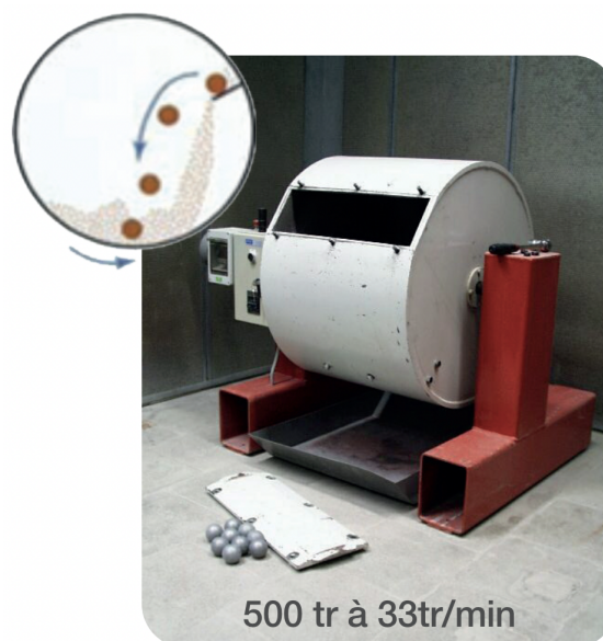
FIGURE 2.13 – Essai Los Angeles [FEREDECO 2023]
