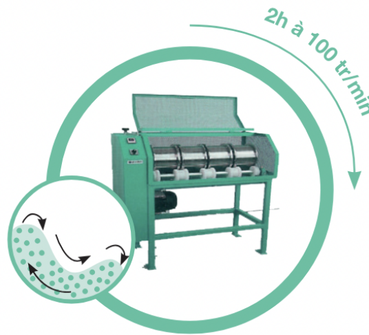
FIGURE 2.16 – Essai Micro-Deval [FEREDECO 2023]
