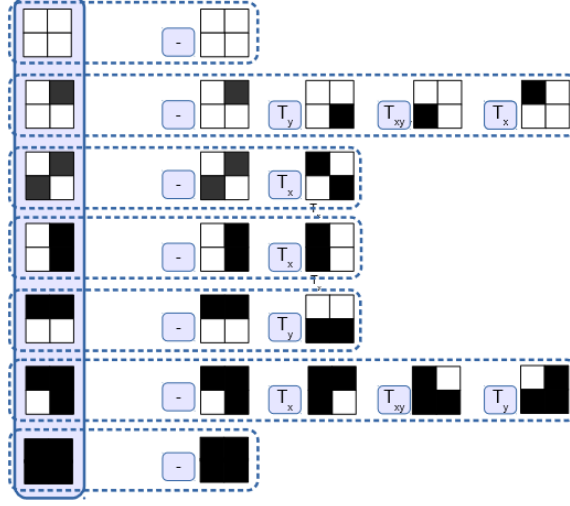
Fig. 1.4: Example of possible symmetric transformation of SADAG on a 2D square brick composed of 4 voxels. Taken from Villanueva et al. [3].
