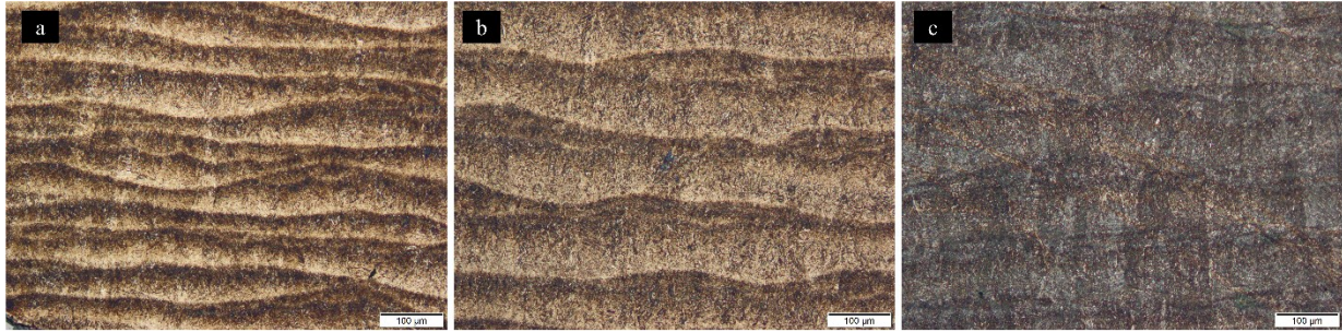
Figure 1: OM micrograph samples post-etching. a) sample treated at 200°C for 10 hours; b) sample treated at 300°C for 10 hours and c) sample treated at 400°C for 10 hours.
