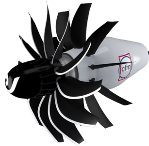
FIGURE 4 – CFM Rise engine concept [14].
