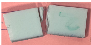
Figure 2.28 – Sample 2 with c/t = 0.05 after fracture.
