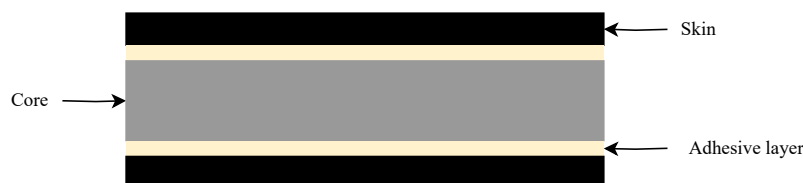
Figure 1.4: Illustration of a sandwich structure.
