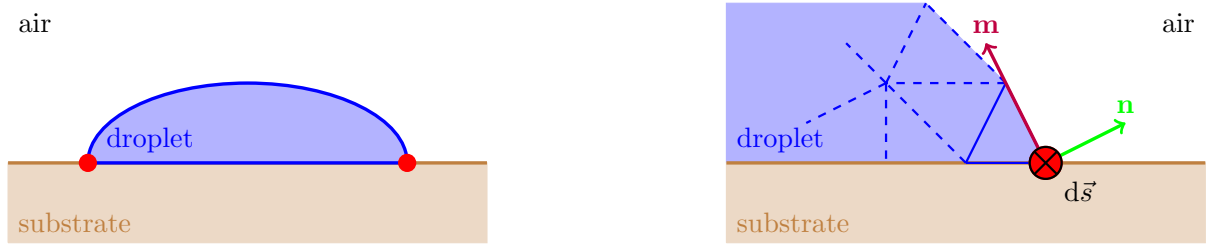
Figure III.3: Representation of the boundary \partial\Gamma_L \equiv \partial\Gamma (red dots) and its tangent vector d\mathbf{s} (noted d\vec{s} in the figure) as well as the vector \mathbf{m} . The figure on the right is a zoom on the right side of the droplet.
