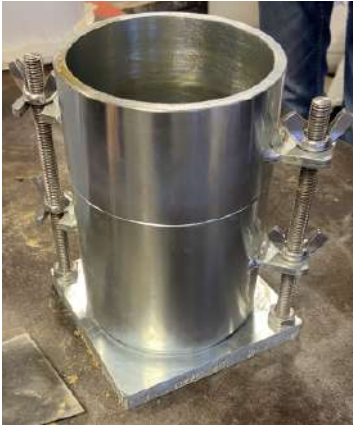
FIGURE 3.9 – Moule Proctor
