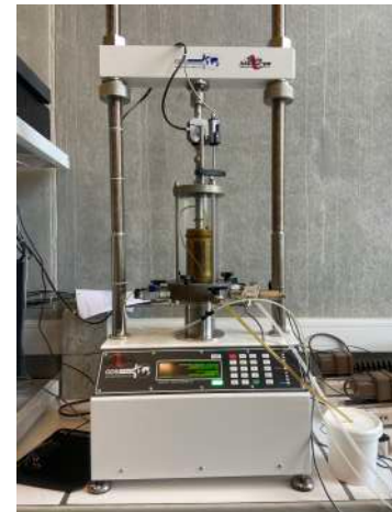
FIGURE 4.17 – Appareil triaxial
