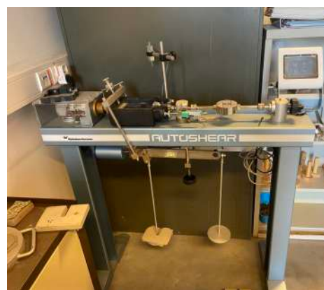
FIGURE 4.14 – Banc de cisaillement
