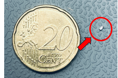
Figure 2.39: Picture of a 100 nF capacitor using 0603 package
