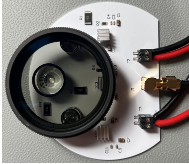
Figure 3.9: Emitter superimposed by the two polarisers uncrossed
