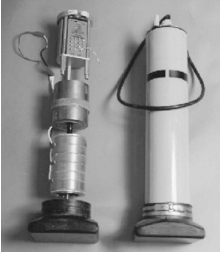
Figure 3: Picture of a Tonpilz acoustic transducer with its piezo stack. Taken from [12] p.10
