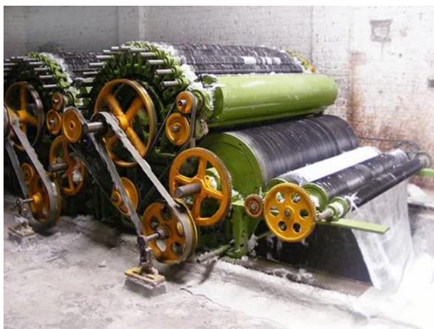
Figure 19. Garnett textile recycling machine (Source: https://www.indiamart.com/proddetail/garnett-machine-14013596412.html )
