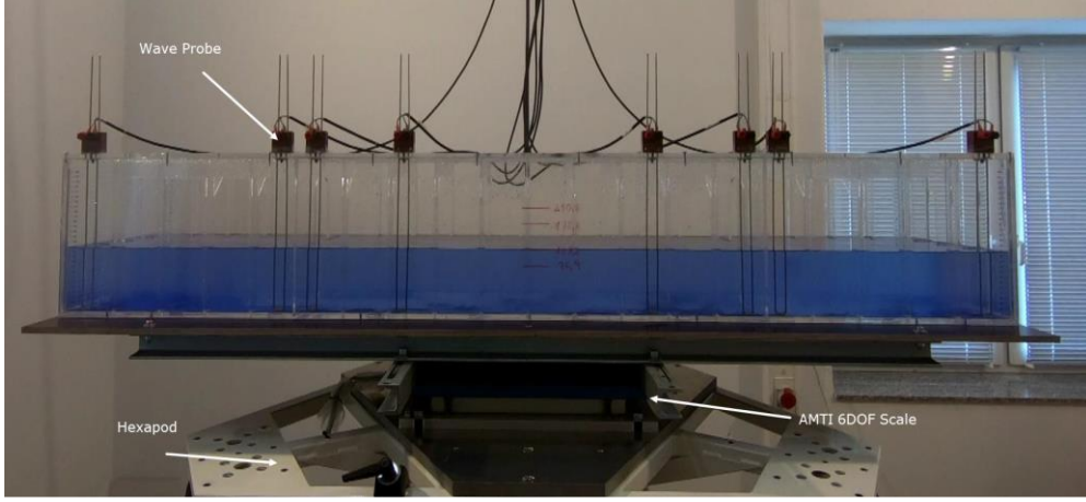
Figure 3-1: Bench Model Test Set-up
