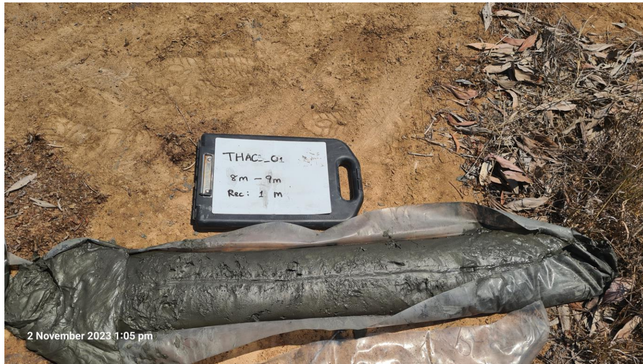
Figure 59: A retrieved sonic drill core.
