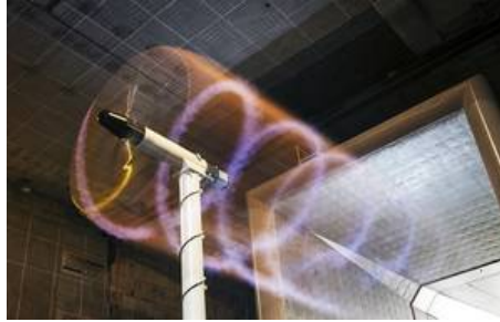
Figure 3.1 – Typical helicoidal flow created at the blade tip, behind a Wind Turbine (Mexico rotor of MexNext project), from [9]
