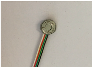
Figure 2.63 – Flush-mounted transducer used to measure reference pressure
