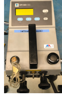
Figure 2.56 – Druck@DPI063 static calibrator in KTH, 100 [Pa] accuracy
