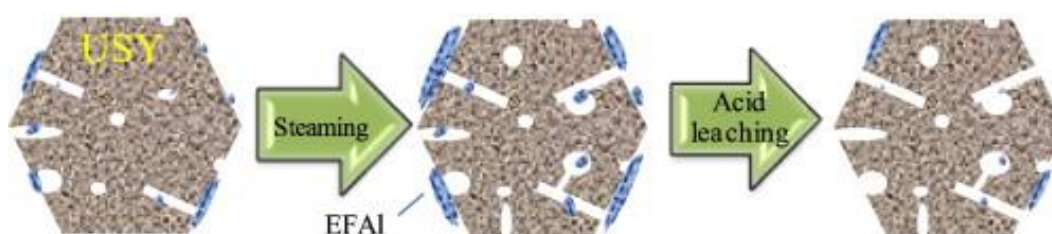
Figure 15. Graphical abstract of the post-synthetic dealumination treatments of Y zeolites (Taken from publication [17])
