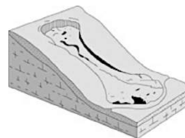
Illustration 6 – Écoulement lent (Source : British Geological Survey)
